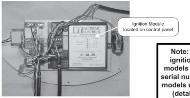
Note: Replacement hot surface ignition module works on all EF models prior to and later than "CF" serial numbers. Direct spark ignition models use a different control board (detailed in following section).
